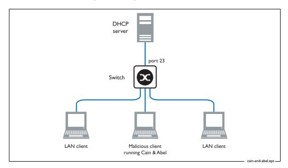
In this scenario, the DHCP server is connected to port 23 on an AT-9924 switch, and three clients are also connected to the AT-9924 switch and receive a valid IP address from the DHCP server. Once the clients have received their DHCP leases, successful L3 connectivity can be verified by pinging from the DHCP server to each client on the LAN.
