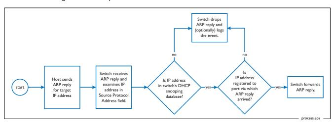
Therefore, ARP security makes it impossible for a host to poison the ARP caches of other hosts, because the switch only forwards ARP packets that have genuine information in the Source Protocol Address field.
